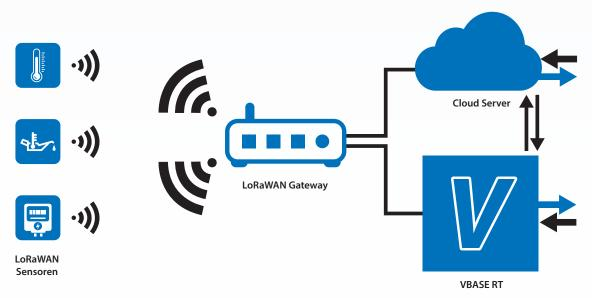
VBASE communicates directly with the LoRaWAN gateway and processes the data from the connected sensors or transfers it to other dedicated systems.
